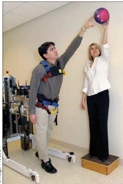
The KineAssist, a novel robotic device, challenges patients who are recovering from stroke or other neurological conditions while reducing the risk of injuries.
